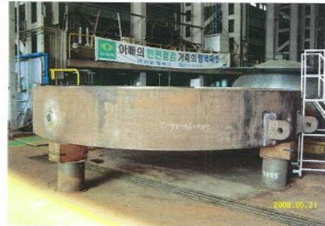
#3B : T/S Cladding & Machining has been completed.
