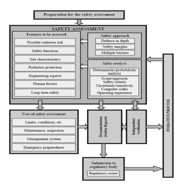
Fig. Overview of Operator's Safety Assessment Process (from GSR-p4)
