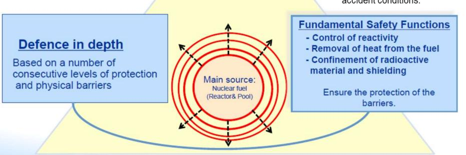
The current implementation of DiD at LWRs comprises 5 levels of protection and 4 physical barriers (fuel matrix, fuel cladding, reactor coolant boundary and containment building) <sup>21</sup>
