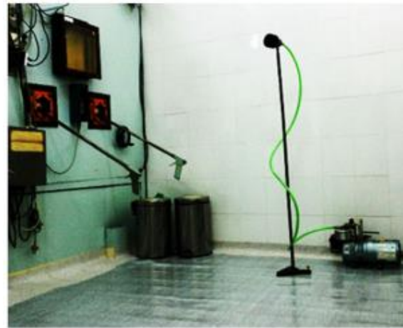
Figure 1. The cartridge holder of the sampling system was settled at the height of 1.5 m from the floor, near the worker's breathing zone.
