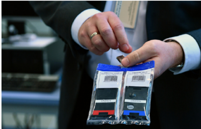
A radiation dosimeter used for individual monitoring in IAEA laboratories. (Photo: D. Calma/IAEA)
