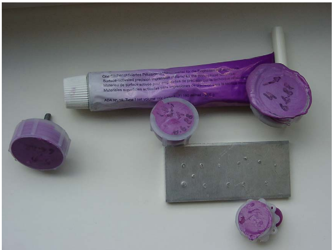
Figure 3: Replica material to determine the dimension of a corrosion spot
