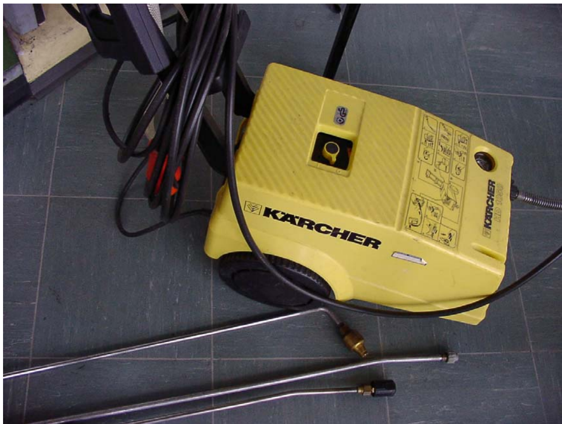
Fig.5: Underwater jet to remove deposits
